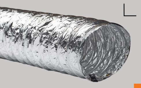
MNI25 is a UL-181 listed and labeled Class 1 non-insulated Air Connector. MNI25 is widely used in the HVAC industry as a supply, return, and exhaust duct in low to medium pressure air conditioning systems, and exhaust applications.
