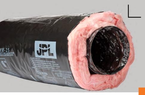
MH25 is a UL-181 Class 1 flexible air duct, manufactured with a heavyduty black polyethylene vapor barrier, which is designed as a supply or return air duct used in manufacturing housing and mobile home installations.
